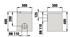
with longitudinal ductile iron grating SW 8 mm, galvanised
