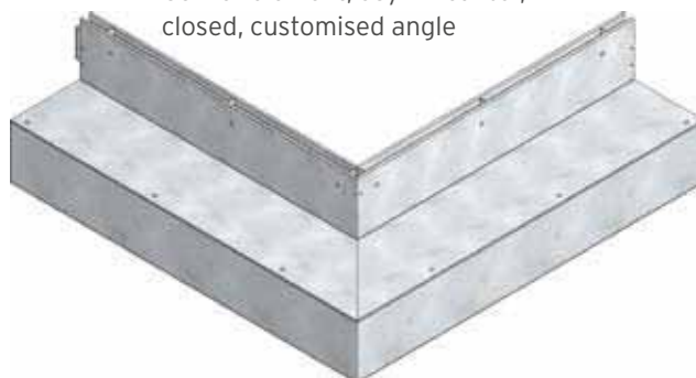
Corner element, asymmetrical, perforated, customised angle
